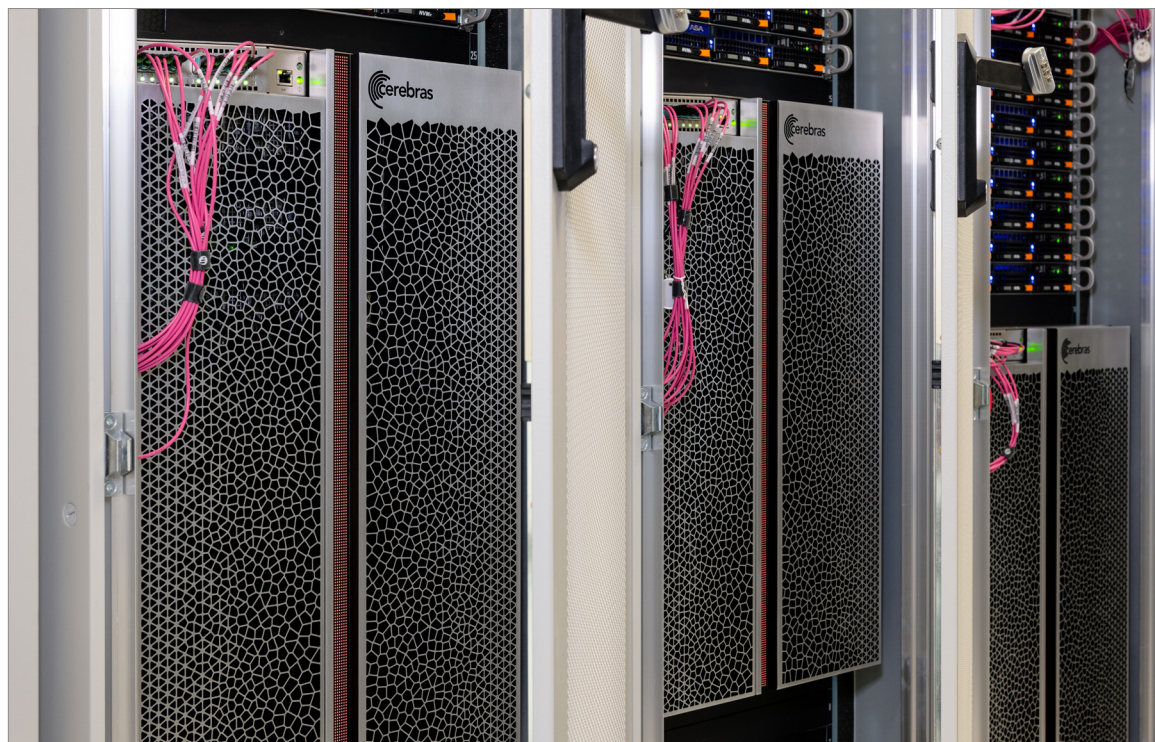
Figure 8: Clusters of CS-2s can run in both model parallel and data parallel modes.
